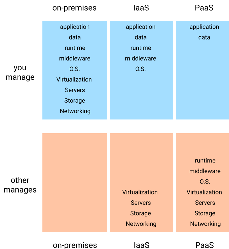
Figure 2.7: Cloud models: a comparison between on-premises, IaaS and PaaS. On the blue zone, assets the developer must manage; on the beige zone, assets the provider manages.
